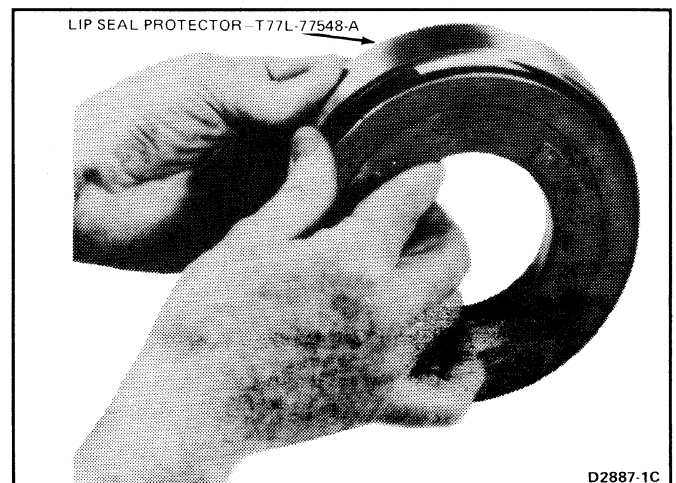
FIG. 52 Installing Forward Clutch Piston and Lip Seal
